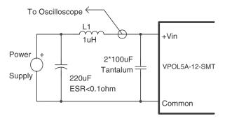
Figure 10. Input Reflected-Ripple Test Setup
