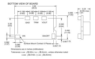
Figure 15 VPOL5A-12-SMT Mechanical Outline Diagram
