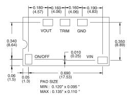
Figure 5. Recommended VPOL5A-12-SMT Footprint (Top View)
