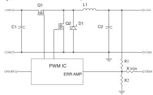
Figure 1. Electrical Block Diagram
