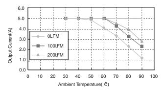
Figure 3. Typal Power Derating for 12V IN 3.36/ut
