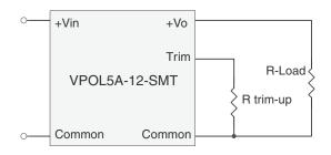
Figure 12. Trim-up Voltage Setup
