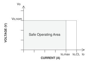
Figure 2. Maximum Output Current Safe Operating Area
