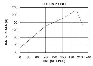
Figure 14 VPOL5A-12-SMT Reflow Profile
