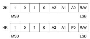
Figure 7-1. Device Address
