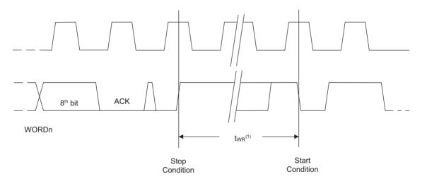
Note: 1. The write cycle time t<sub>WR</sub> is the time from a valid Stop condition of a write sequence to the end of the internal clear/write cycle.
