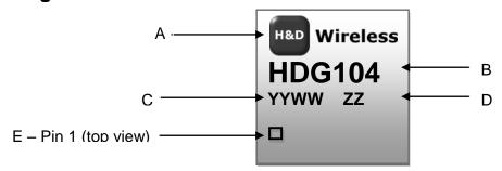
Figure 6.2: HDG104 QFN package marking.
