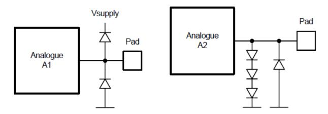
Figure 3-5: Schematics of analogue inputs A1 and A2
