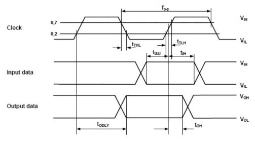
Figure 3-2: SDIO timing diagram (high speed mode)
