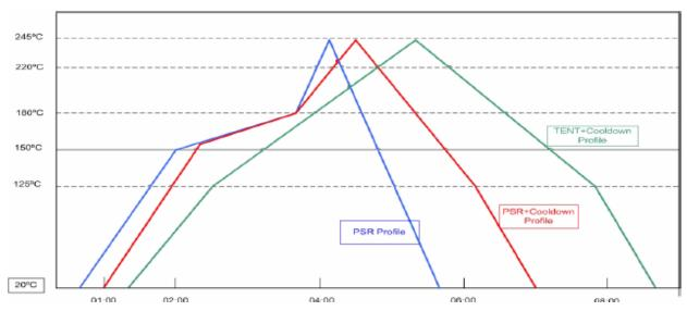
Figure 5-5: Reflow Temperature Profile.
