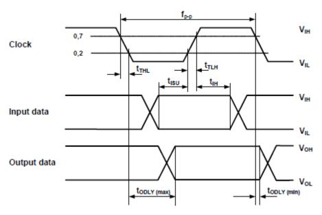
Figure 3-1: SDIO/SPI timing diagram (default mode)
