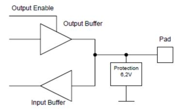
Figure 3-4: Function schematics of the I/O input pad configuration.
