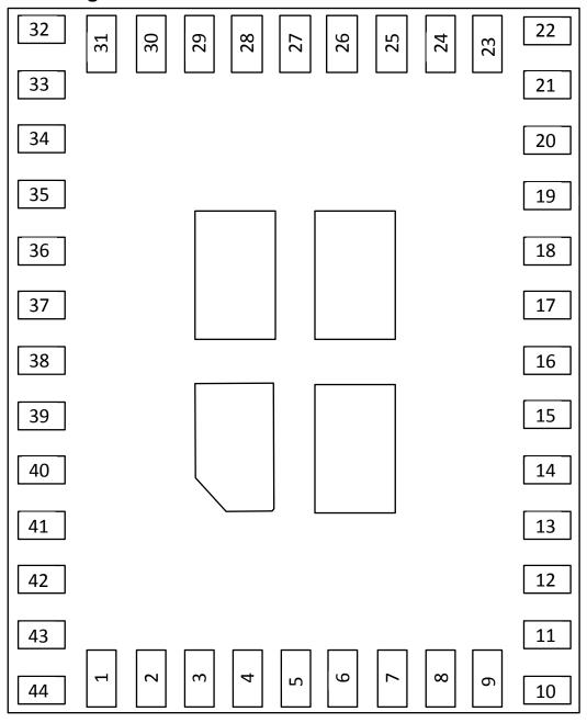
Figure 4-1: Package pin out. Top view
