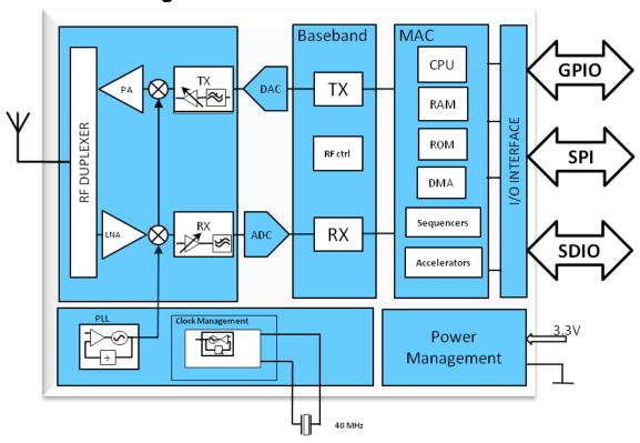
Figure 2.1: Block diagram.
