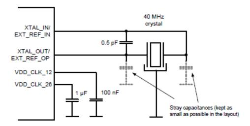
Figure 5-1: Reference clock setup
