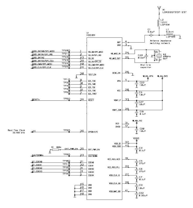
Figure 5-6: Reference design schematic.
