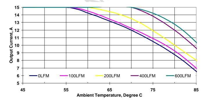
Figure 16. Thermal Derating Curves. Vin=14V, Vout=5.0V
