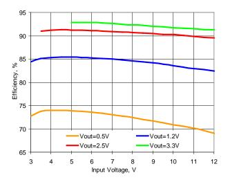
Figure 6. Efficiency vs. Input Voltage. lout=15A
