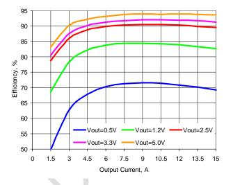
Figure 4. Efficiency vs. Load. Vin=12V
