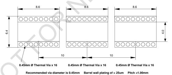
Figure 22. Recommended PCB Layout for Multilayer PCBs
