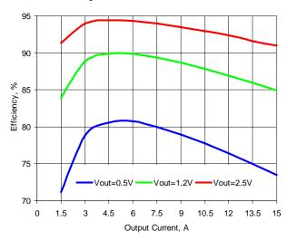
Figure 2. Efficiency vs. Load. Vin=3.3V
