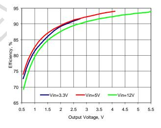
Figure 5. Efficiency vs. Output Voltage, lout=15A
