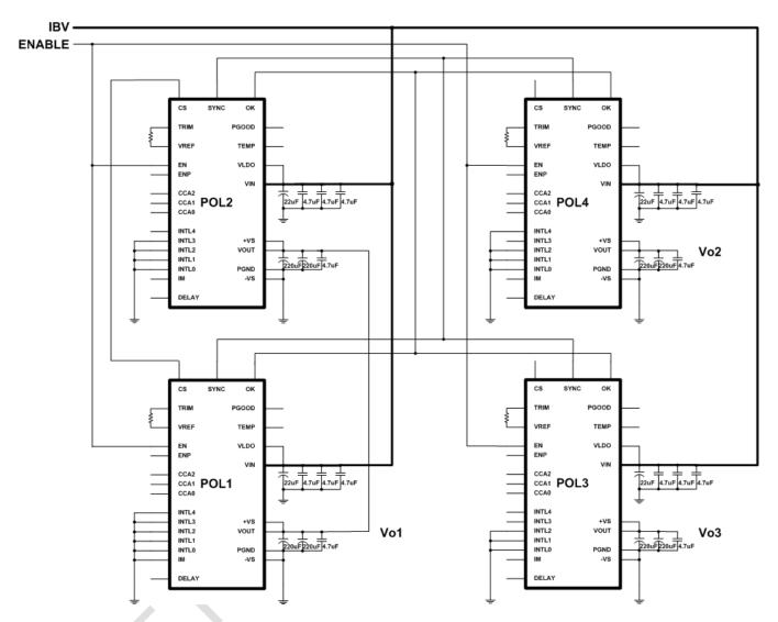
Figure 17. Complete Schematic of Application with Three Independent Outputs. Intermediate Bus Voltage is from 8V to 14V.
