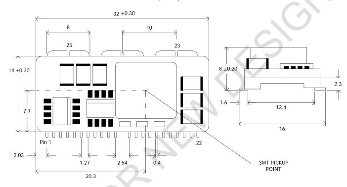
Figure 20. Mechanical Drawing
