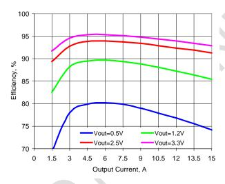
Figure 3. Efficiency vs. Load. Vin=5V
