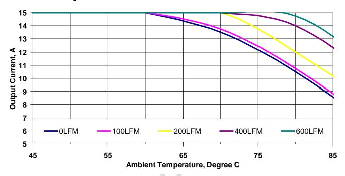
Figure 15. Thermal Derating Curves. Vin=12V, Vout=5.0V
