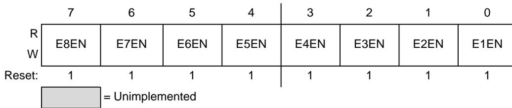
**Figure 17. Electrode Channel Enable Mask Position Register**
