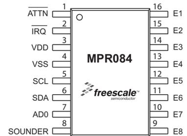
Figure 1. Pin Connections
