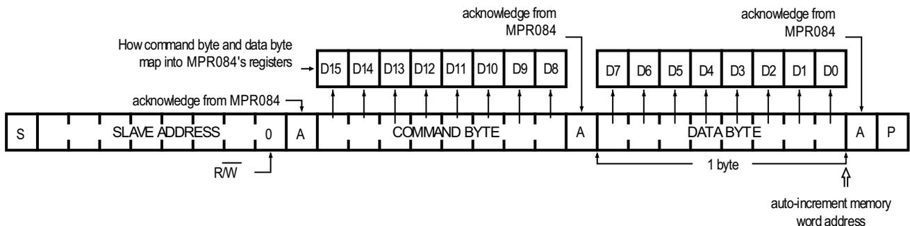
**Figure 11. Command and Single Data Byte Received**
