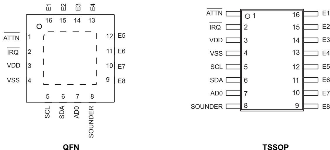
**Figure 3. Package Pinouts**
